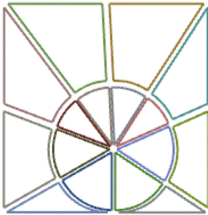
Fig. 23. Subdivision of regular quadrilateral element with BTSM with source point at (0.075, -0.4) .
