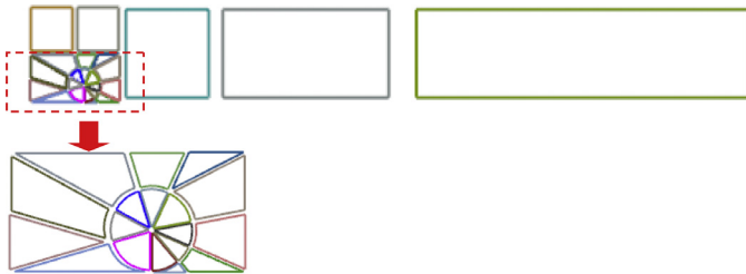
Fig. 25. Subdivision of slender quadrilateral element with BTSM with source point at (-0.85, -0.65) .
